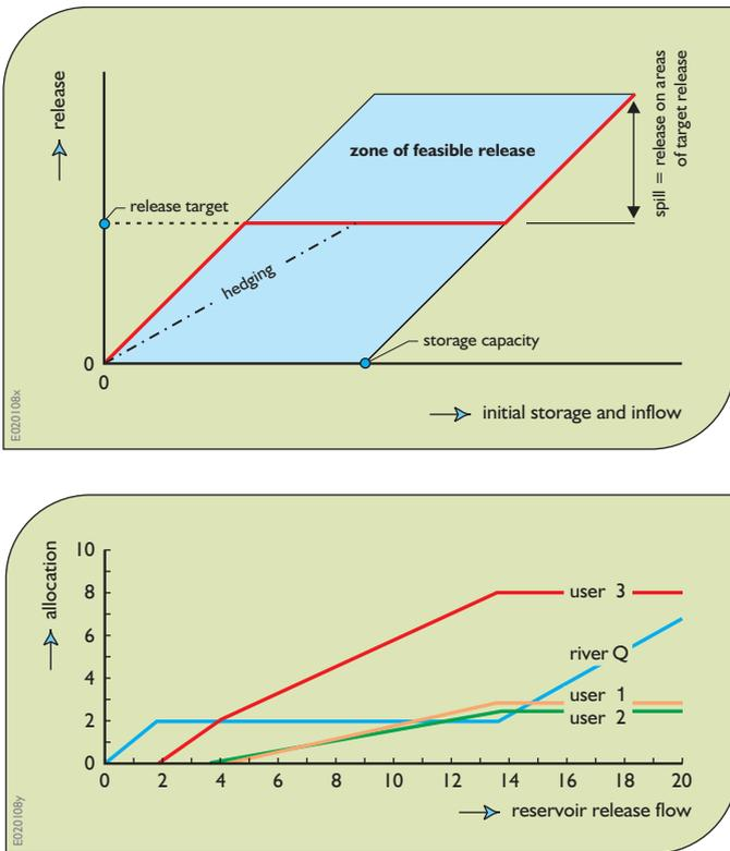
**Figure 3.3.** Policy defining the reservoir release to be made as a function of the current storage volume and current inflow and the reservoir release allocation policy for the river flow downstream of the reservoir. The blue zone in the reservoir release policy indicates the zone of feasible releases. It is physically impossible to make releases represented by points outside that blue zone.
