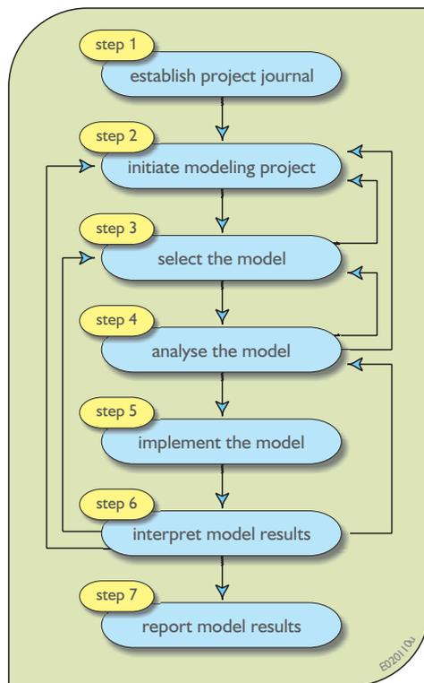
**Figure 3.8.** The modelling project process is an iterative procedure involving specific steps or tasks.
